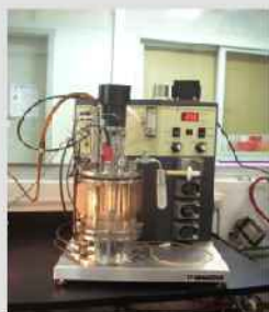
2.5 l Fermentor, with 1.5 l working volume
