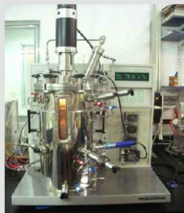
20 l Fermentor, with 15 l working volume
