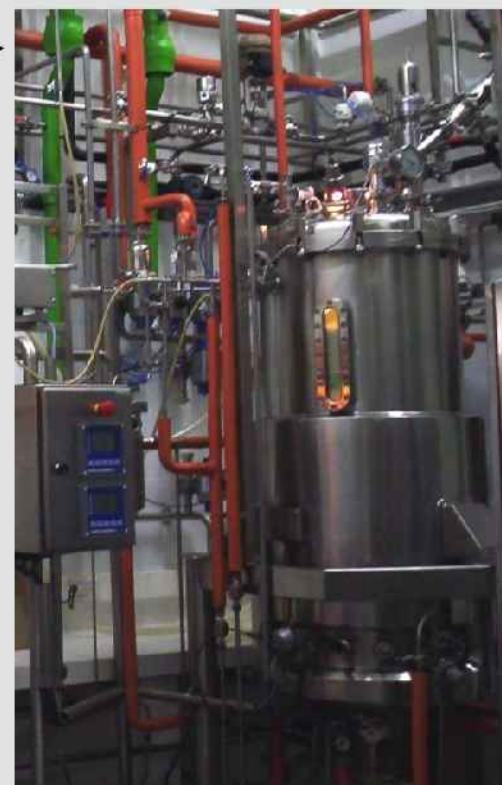
370 l Fermentor, with 300 l working volume
